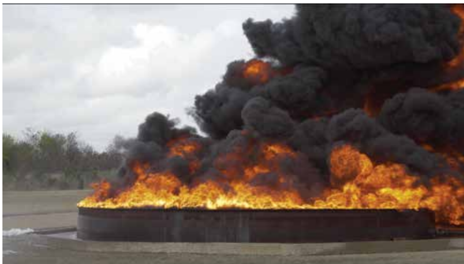
PRE-BURN PETROLEUM STORAGE TANK SIMULATOR 42 FT (128 m) DIAMETER
